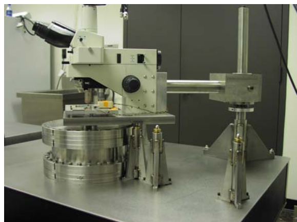
Fig. 1. The new microbeam irradiation station. On the right is the pivot arm for moving the microscope between the online and off-line positions. It will also be used to move the SEIM online and off line. The stands in the lower middle and right are to support the microscope when in the off-line position. The voice coils stage is in place on the microscope.
