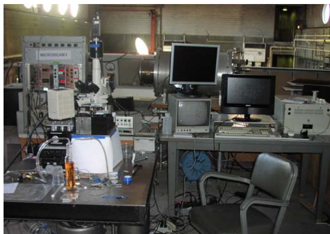
Fig. 2 The original microbeam irradiation station moved to the floor above the original microbeam room (normally storage) for use in testing the stand alone microbeam system. One of the permanent magnet quadrupole triplets is inside the white enclosure (to keep it clean) in the middle of the table on the left.
