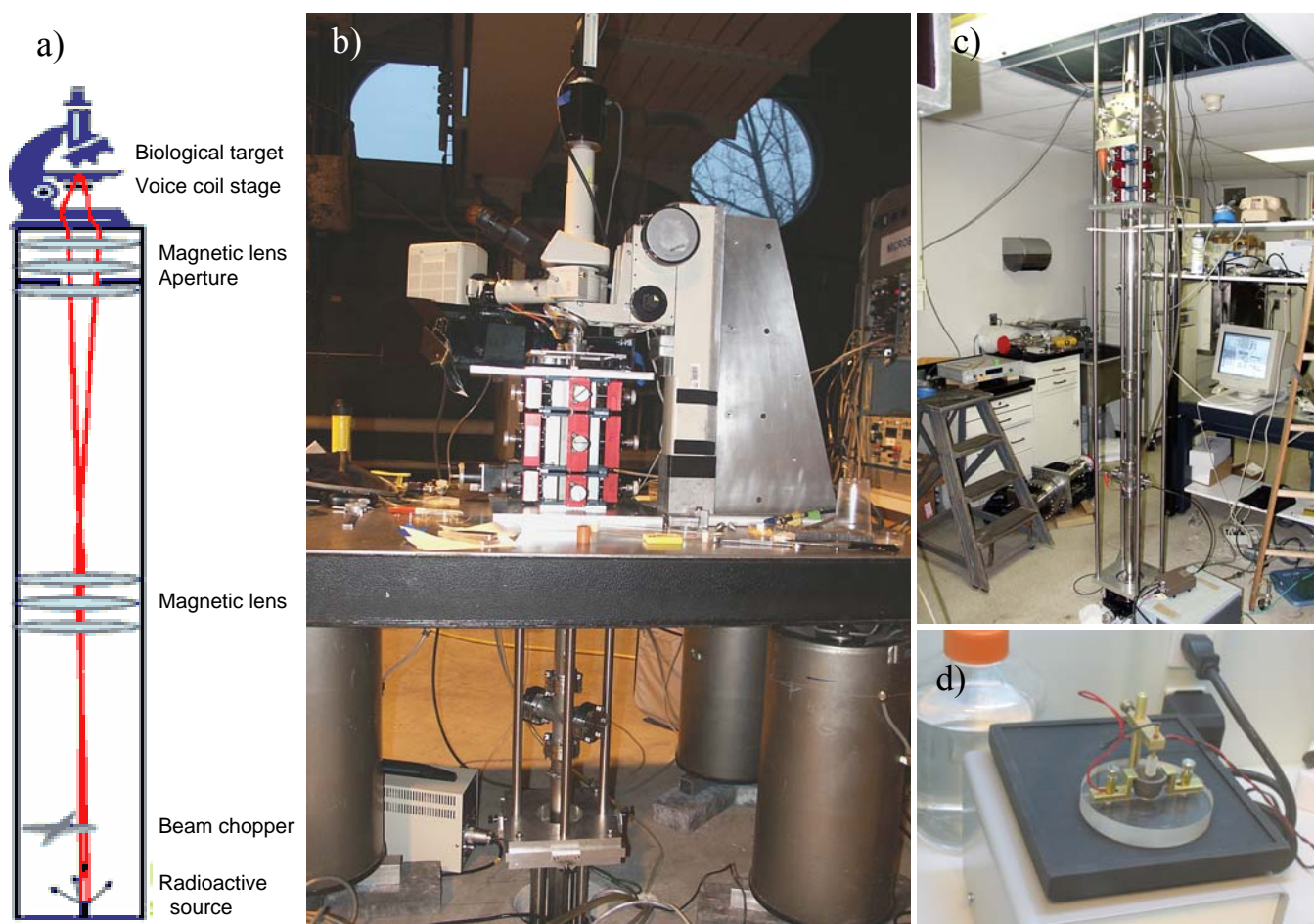
The new RARAF stand-alone microbeam: a) Diagram of the stand-alone microbeam's principle elements. A small, high specific-activity \alpha -emitter is used as a source. A compound magnetic lens, consisting of 24 permanent magnets arranged in two quadrupole triplets, focuses the emitted \alpha -particles. The first triplet is placed 2 m above the source, with a second identical triplet placed 2 m above the focal plane of the first. The cells to be irradiated are placed at the image plane on a voice coil stage. The endstation consists of the voice coil stage and a microscope with a particle detector mounted on the objective lens. b) The microbeam endstation and immediately below it the upper magnetic quadrupole triplet. c) The source holder (near floor) and the lower quadrupole triplet. d) A system for electroplating polonium onto the end of a wire, to create the 1-mm diameter, \alpha -particle source.
