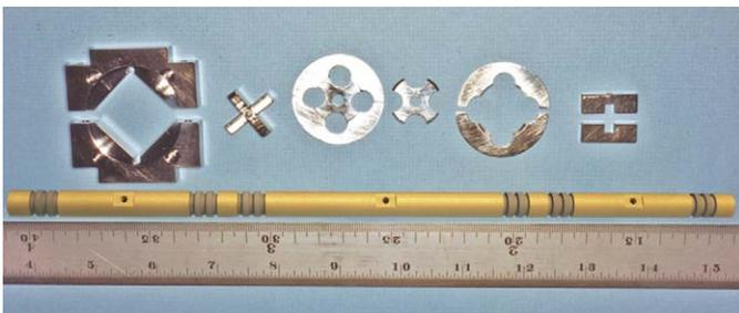
**Fig. 3.** Photograph of the electrostatic lens components (L–R): V-blocks used to clamp the lens rods; assembled cross spacer; field shaping disc; inner (cross) and outer (ring) parts of the field shaping disc; and two halves of a cross spacer. Below these components is one of the ceramic rods for a quadrupole triplet.
